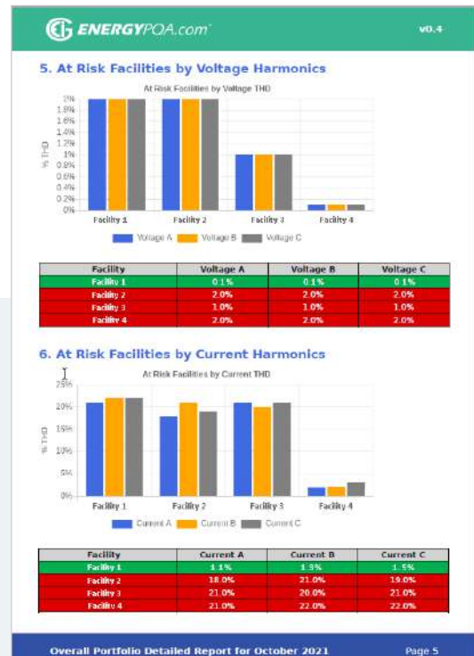
At-risk Facilities Based on Voltage and Current Harmonics
